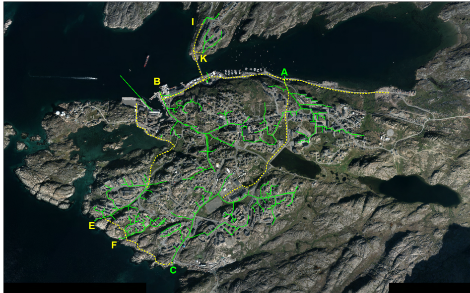
Figure 77: The existing and planned sewer system in Sisimiut. The green line shows the existing sewage lines, whereas the yellow lines indicates the planned ones. The capital letters indicate sewage outlet points. The plan is, that outlet points indicated in yellow letters shall be removed, whereas the green ones will be maintained. Ulkebugten outlet is “A” and the recommend alternative outlet site is the Natreno outlet “C”, and then with a sewage treatment plant installed here
