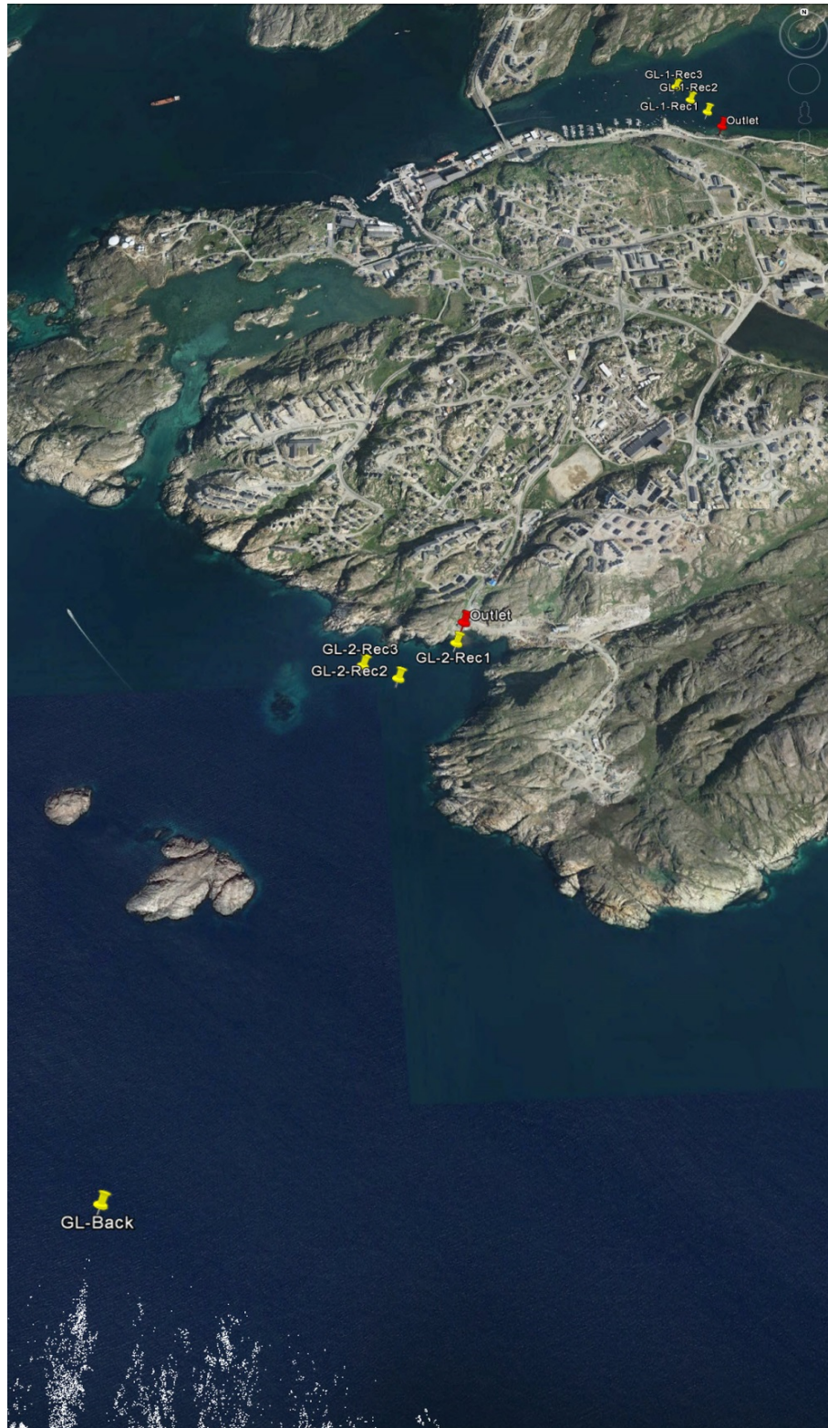
Figure 18: Sampling sites used in 1st round in Sisimiut. The Ulkebugt sewage line outlet is in the upper right corner, and the Natreno sewage line outlet is shown in the middle of the picture
