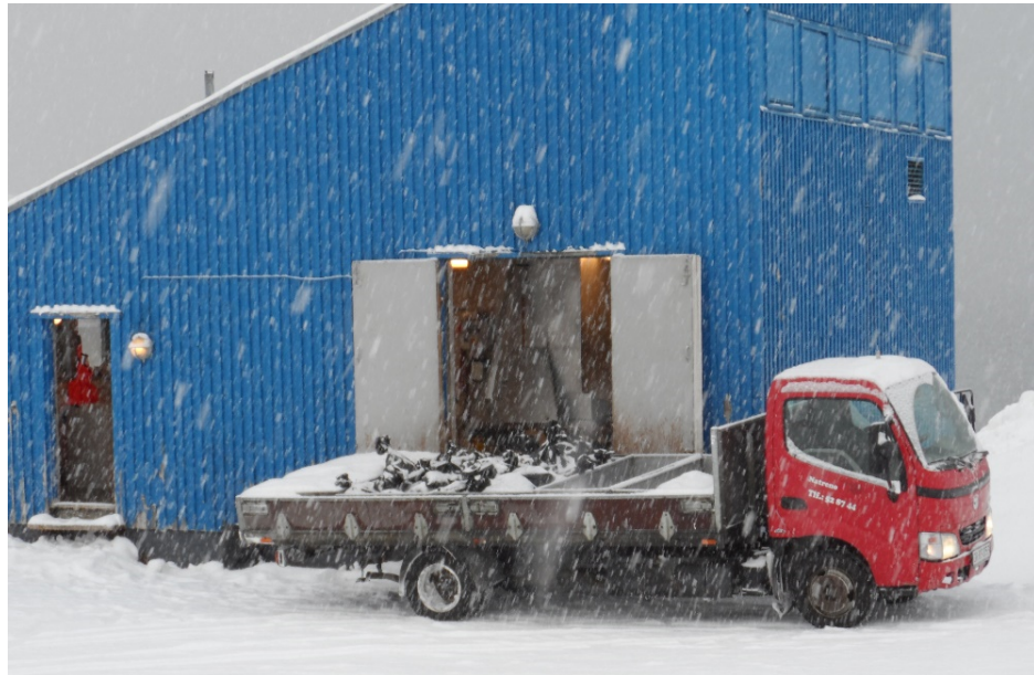
Figure 9: In parts of Sisimiut, the removal of the black wastewater involves a man-and-truck-based collection of the plastic bags which subsequently are emptied and the contents discharged to sea, as here at the Natreno site
